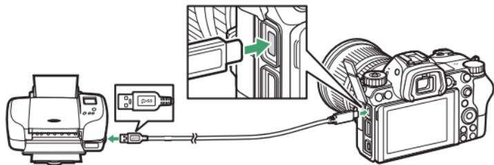
When the camera and printer are turned on, a welcome screen will be displayed, followed by a PictBridge playback display.
