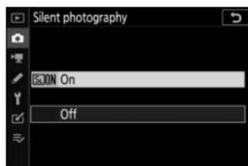
An icon is displayed while silent photography is in effect. In release modes other than **Continuous H (extended)**, the display will briefly go dark when the shutter is released to signal that a photo has been taken.
