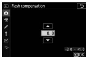
Normal flash output can be restored by setting flash compensation to  $\pm 0.0$ . Flash compensation is not reset when the camera is turned off.
