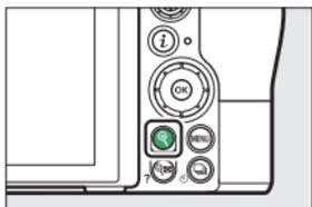
When the subject is in focus, the focus point will light green and the in-focus indicator (●) will appear in the display.
