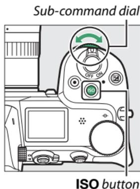
When auto ISO sensitivity control is enabled, the shooting display will show **ISO AUTO** and control panel **ISO-A**. When sensitivity is altered from the value selected by the user, the altered value is shown in the display.
