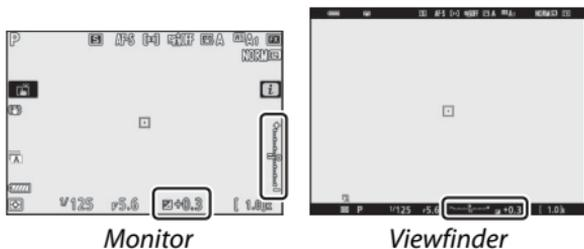
Normal exposure can be restored by setting exposure compensation to  $\pm 0$ . Exposure compensation is not reset when the camera is turned off.
