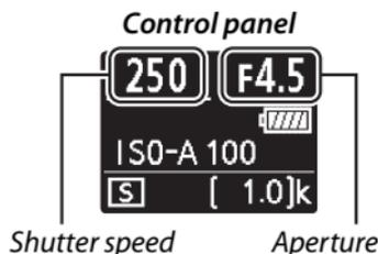
Shutter speed and aperture can be locked at the selected settings.
