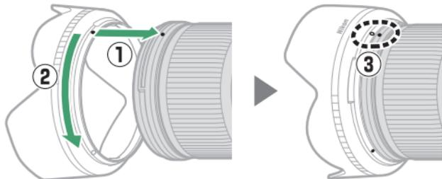
When attaching or removing the hood, hold it near the ● symbol on its base and avoid gripping it too tightly. The hood can be reversed and mounted on the lens when not in use.
