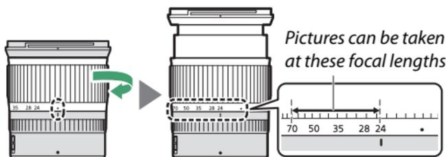
To retract the lens, rotate the zoom ring in the opposite direction, stopping when you reach the (●) position on the focal length scale.
