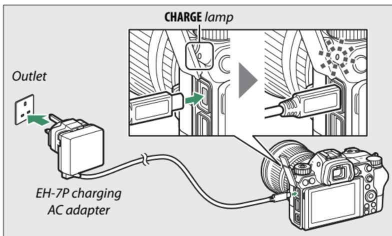
The camera **CHARGE** lamp lights amber while charging is in progress and turns off when charging is complete. Note that although the camera can be used while connected, the battery will not charge and the camera will not draw power from the charging AC adapter while the camera is on.
