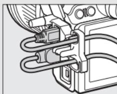
*HDMI cable and USB cable used simultaneously*
