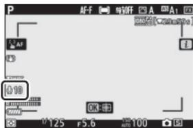
If the sound level is displayed in red, the volume is too high. Reduce microphone sensitivity.
