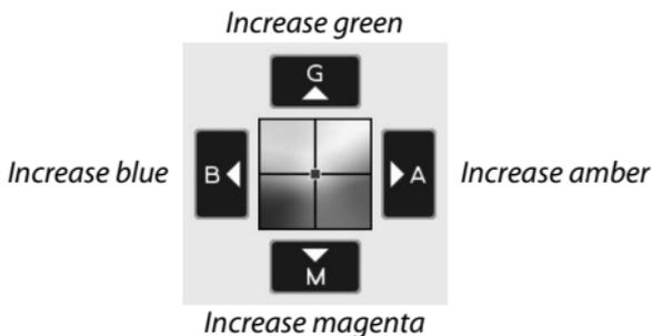
Tap the arrows in the display or use the multi selector to fine-tune white balance. Press
