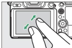
To “zoom out” to a thumbnail view, use a pinch gesture in full-frame playback. Use pinch and stretch to choose the number of images displayed from 4, 9, and 72 frames.
