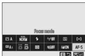
At default settings, the focus mode can also be selected by holding the **Fn2** button and rotating the main command dial ( 24).
