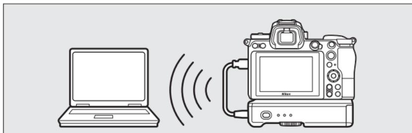
Use the WT-7 for connection to Ethernet networks and for more reliable connections to wireless networks. With Camera Control Pro 2 (available separately), the camera can be controlled remotely and pictures saved directly to the computer as they are taken.
