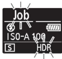
If **On (series)** is selected, HDR will only turn off when **Off** is selected for HDR mode; if **On (single photo)** is selected, HDR turns off automatically after the photograph is taken.
