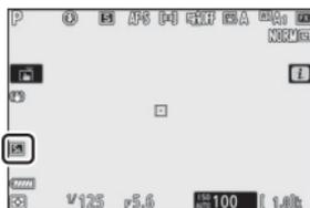
Enabling silent photography changes the frame advance rates for continuous release modes (87) and disables some features, including the flash, long exposure noise reduction, and flicker reduction.
