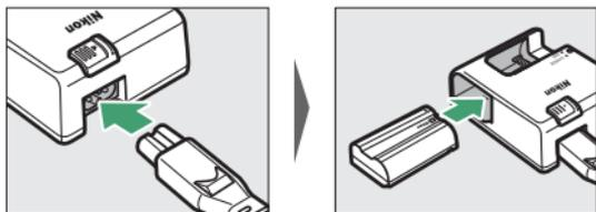
The **CHARGE** lamp will flash while the battery charges. An exhausted battery will fully charge in about two hours and 35 minutes.
