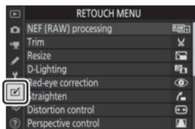
The options in the retouch menu are used to create trimmed or retouched copies of existing pictures. The retouch menu is only displayed when a memory card containing photographs is inserted in the camera.
