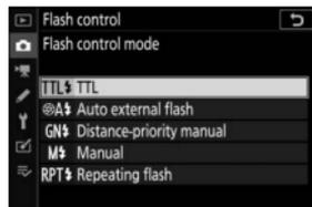
**control mode** item in the photo shooting menu (in the case of the SB-5000, these settings can also be adjusted using the controls on the flash unit). The options available vary with the flash used, while the options displayed under **Flash control mode** vary with the mode selected. Settings for other flash units can only be adjusted using flash unit controls.
