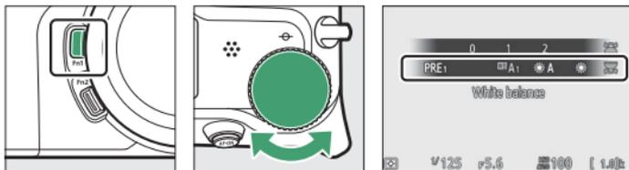
When **WB A (Auto)**, **☀ (Fluorescent)**, **🌡 (Choose color temperature)**, or **PRE (Preset manual)** is selected, you can choose a sub-option by holding the **Fn1** button and rotating the sub-command dial.
