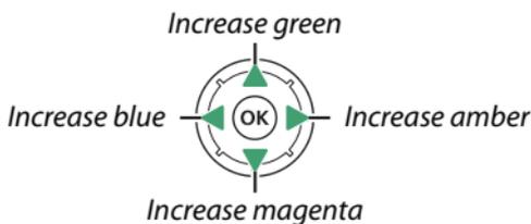
Note that monitor color balance can only be adjusted when the monitor is the active display; it cannot be adjusted in the “viewfinder only” monitor mode or when your eye is to the viewfinder. Monitor color balance applies only to the shooting, playback, and menu displays; pictures taken with the camera are not affected.
