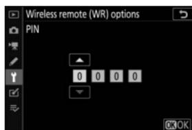
Regardless of the option selected for **Link mode**, signals from paired wireless remote controllers will always be received by the WR-R10. Users of the WR-1 wireless remote controller will need to select pairing as the WR-1 link mode.
