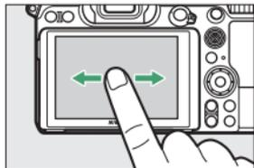
In full-frame view, touching the bottom of the display brings up a frame-advance bar. Slide your finger left or right over the bar to scroll rapidly to other pictures.
