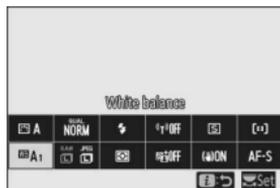
At default settings, white balance can also be selected by holding the **Fn1** button and rotating the main command dial (📖 24).
