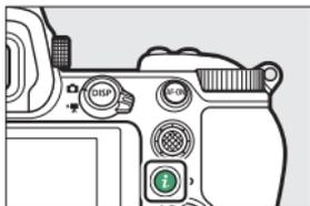
Highlight items using the multi selector and press **OK** to view options, then highlight an option and press **OK** to select it and return to the *i* menu (to exit to the previous display without changing settings, press the *i* button).
