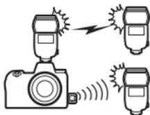
flash unit mounted on the camera accessory shoe. Before proceeding, establish a wireless connection between the radio-controlled flash units and the WR-R10 (📖 366). If an SB-500 is mounted on the camera accessory shoe, select **Optical/radio AWL for Flash control > Wireless flash options** in the photo shooting menu; with other flash units or the SU-800, this option is selected automatically.
